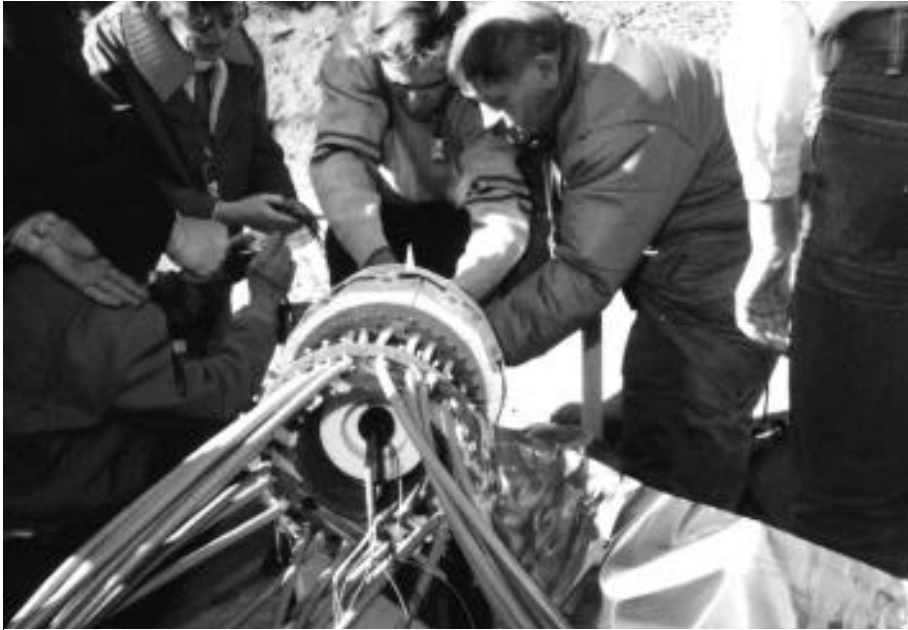
Preparations in Ancho Canyon, Los Alamos in September 1993 for a shot to measure the critical field of high-temperature superconductors.
