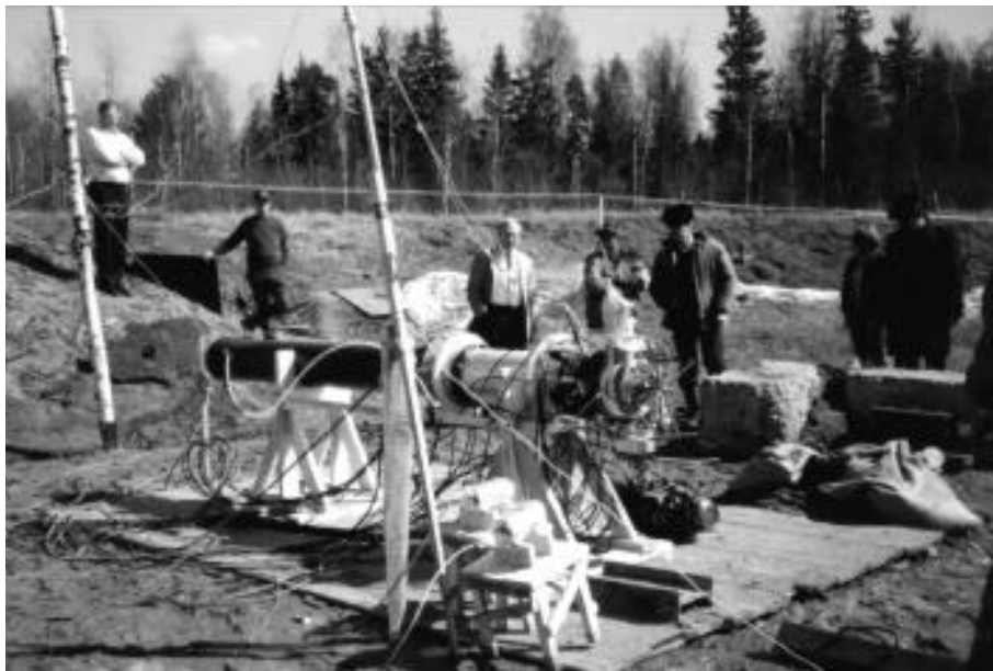
A flux compression generator is on its side at Chernyshev’s firing site at Arzamas-16 in April 1994 and is being prepared to measure the properties of magnetized plasmas.
